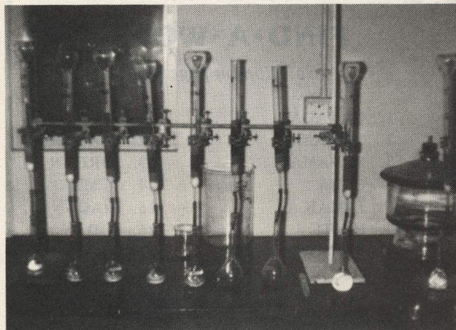
Leaching tubes used to extract elements found in peat samples, at Ministry of Agriculture.
